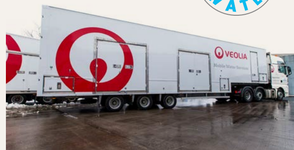
Mobile Water Services containerized RO mobile unit more than 40m 3 /hr capacity
